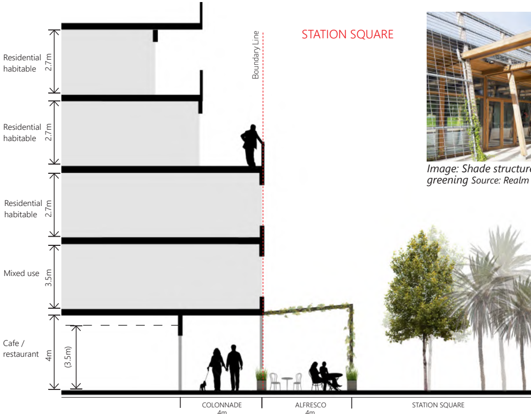
Figure 25: Section 4 - Station Square
