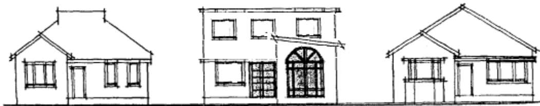
Figure 10 – New development (centre) ignores existing patterns and uses a flat roof, horizontally proportioned window, an uncharacteristically large arched window, and a double leaf door.
