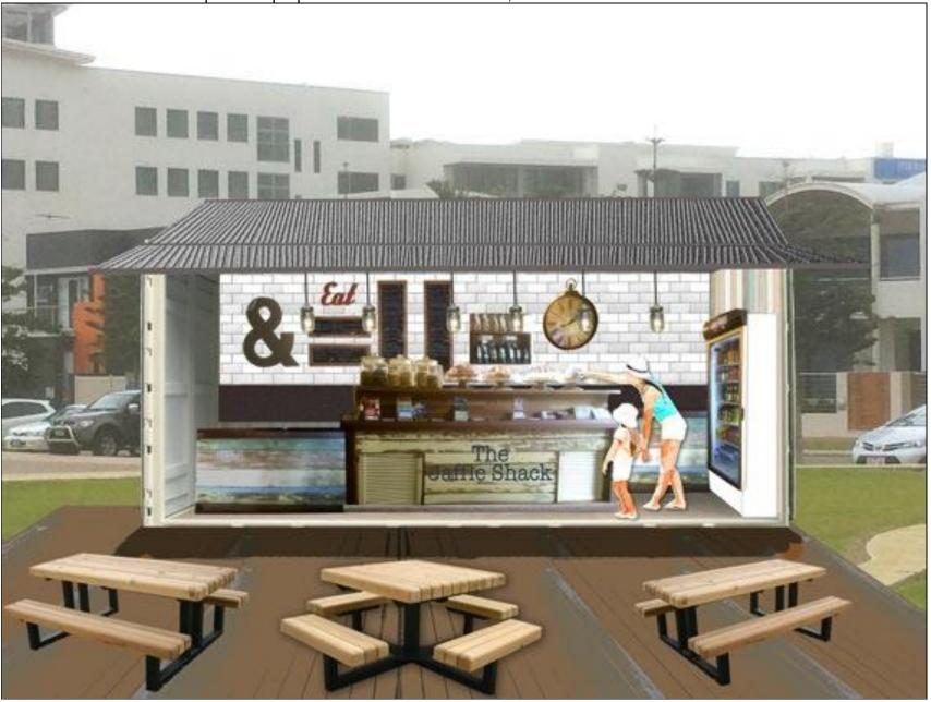
The Cafe is to be alfresco focused and contained within a side opening sea container. The container to be fully clad and roofed so as to disguise the fact it is a sea container and give the appearance of a shack.
