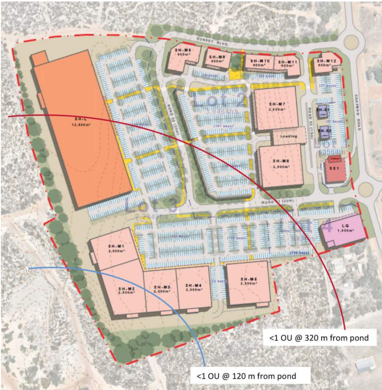
Figure 6. Odour Distances from WWTP
