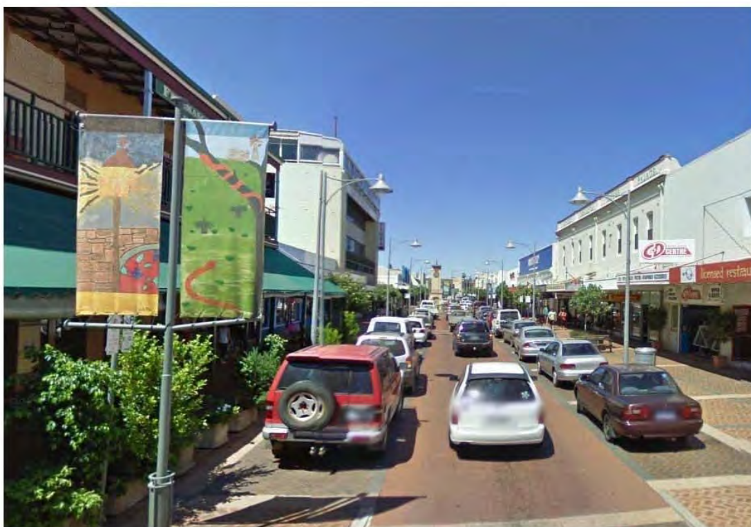
Example of main street Geraldton showing active frontages, urban street furniture, features to encourage pedestrian use (i.e. coverings, wide pavements & different use of materials) and low speed environment for vehicles
