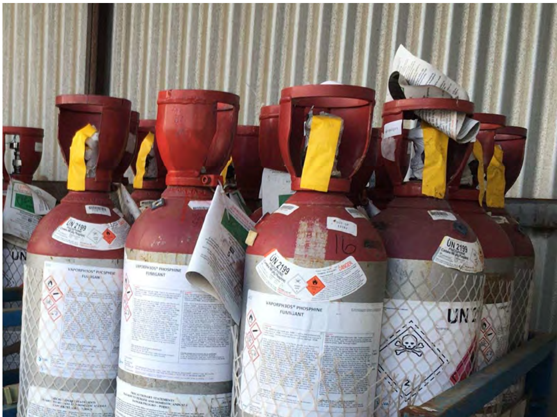
Photo 24 – *VaporPhos cylinders showing labelling and valve protection
