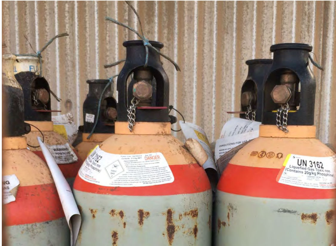
Photo 25 – *EcoFume cylinders showing caps and labelling
