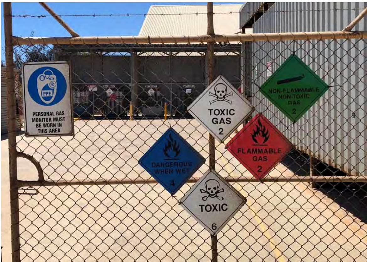
Photo 12 – *DG placards / diamonds and signage on the front gate of the DG compound
