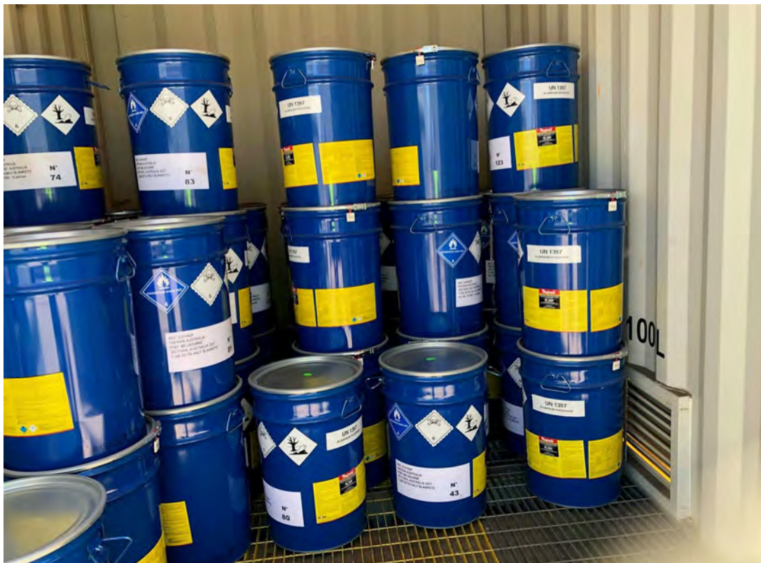
Photo 6 – *Labelling and stacking of AIP drums in Store PS2
