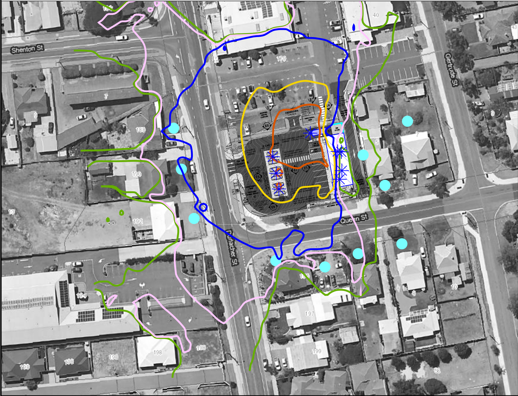
Figure 4-2 Scenario 2: Night Time Noise Ground Floor (1.5m AGL), dB LA1
