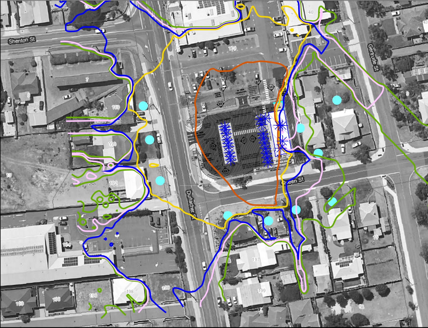
Figure 4-3 Scenario 3: Night Time Noise Ground Floor (1.5m AGL), dB L Amax
