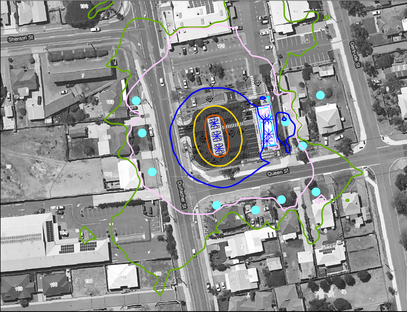
Figure 4-1 Scenario 1: Night Time Noise Ground Floor (1.5m AGL), dB LA10
