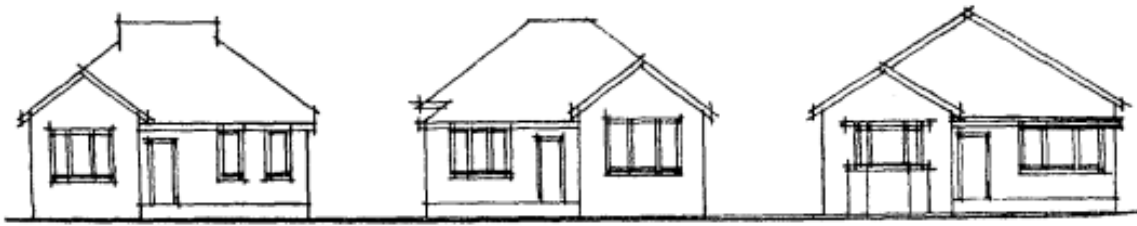
Figure 9: Existing development has a repetition of built form, with similar shapes and scale, consistent roof line and vertically proportioned windows and single leaf doors.
