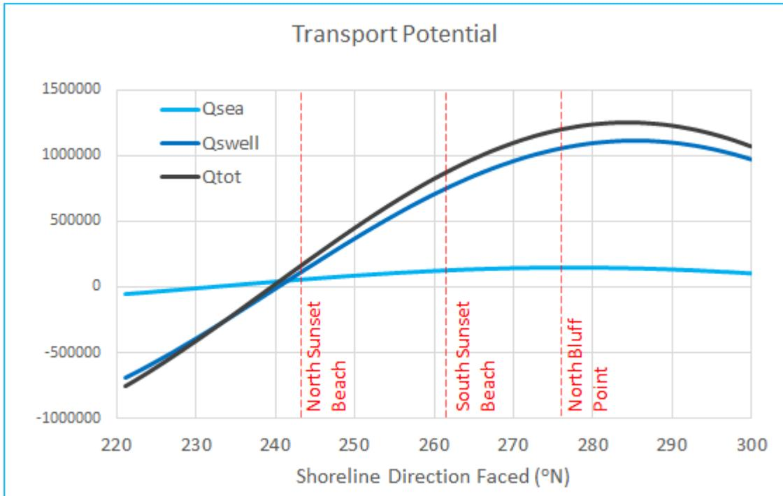
**Figure B-17: Variation of Alongshore Sediment Transport Potential with Shore Direction**
