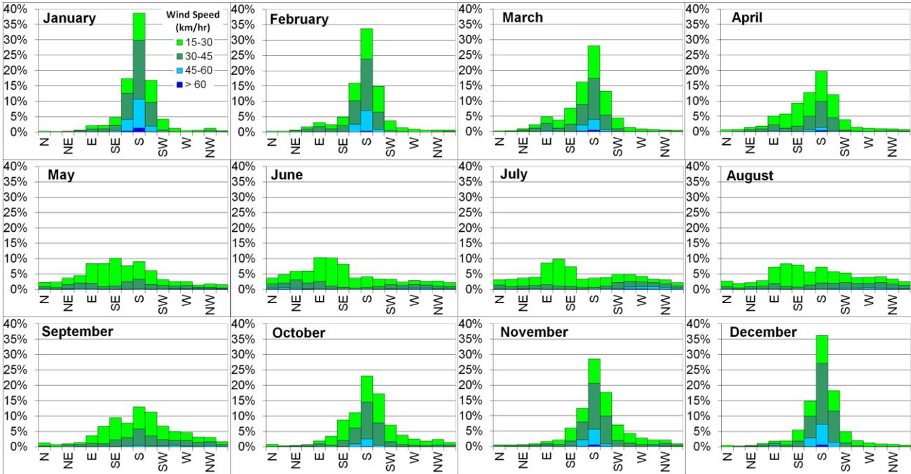
Figure A-2: Monthly Wind Speed and Direction Frequencies (Outer Channel)
