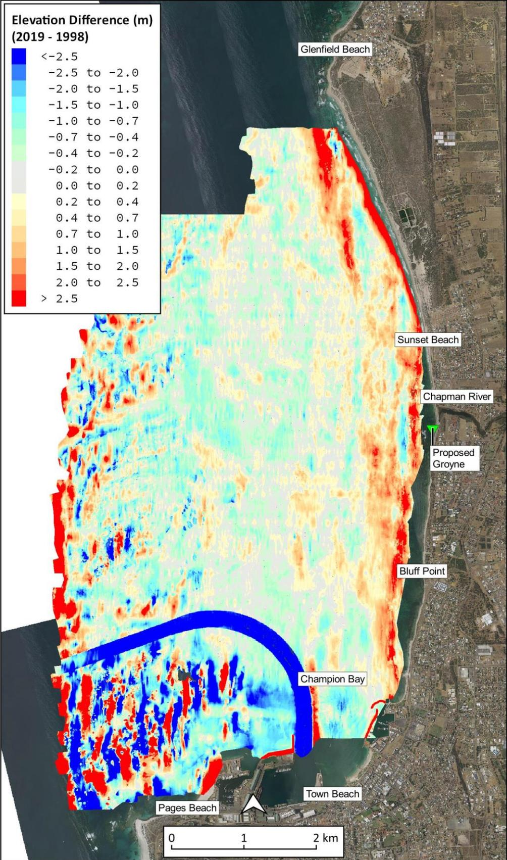
**Figure B-4: Elevation Difference Analysis – 1988 Single Beam Survey to 2016 LIDAR**
