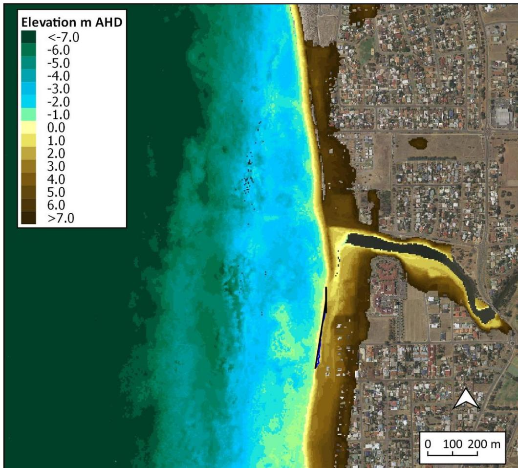
**Figure B-5: Bathymetry and Nearshore Topography from 2016 LIDAR**
