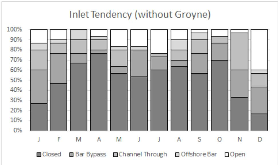
**Figure 3-2: Inlet Tendency Due to Tide and Alongshore Transport Simulation for 10,000 m<sup>3</sup>/yr alongshore transport**
