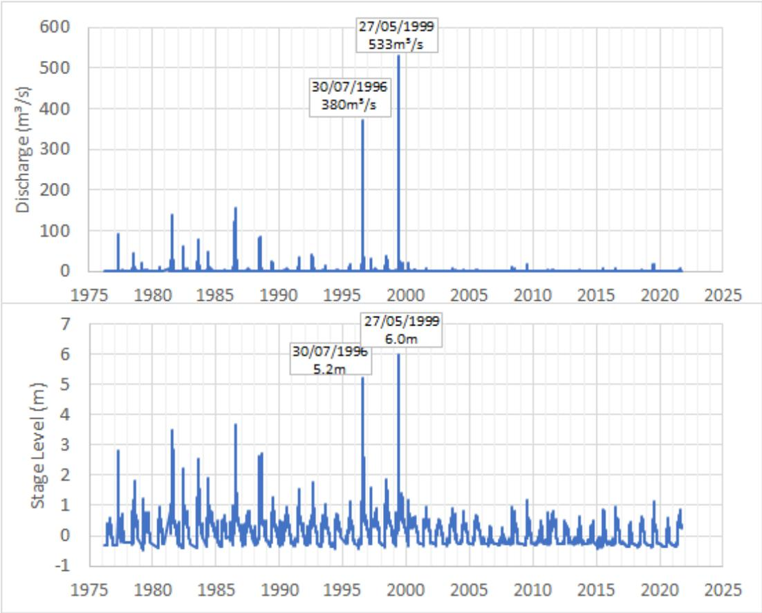
Figure A-11: Chapman River Discharge (Top) and Stage Level (Bottom) at Utakarra
