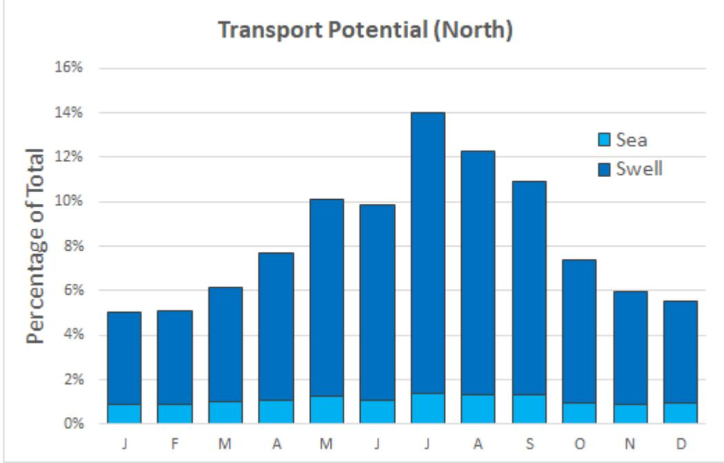
Figure B-16: Seasonal Variation of Alongshore Sediment Transport Potential (Scaled)
