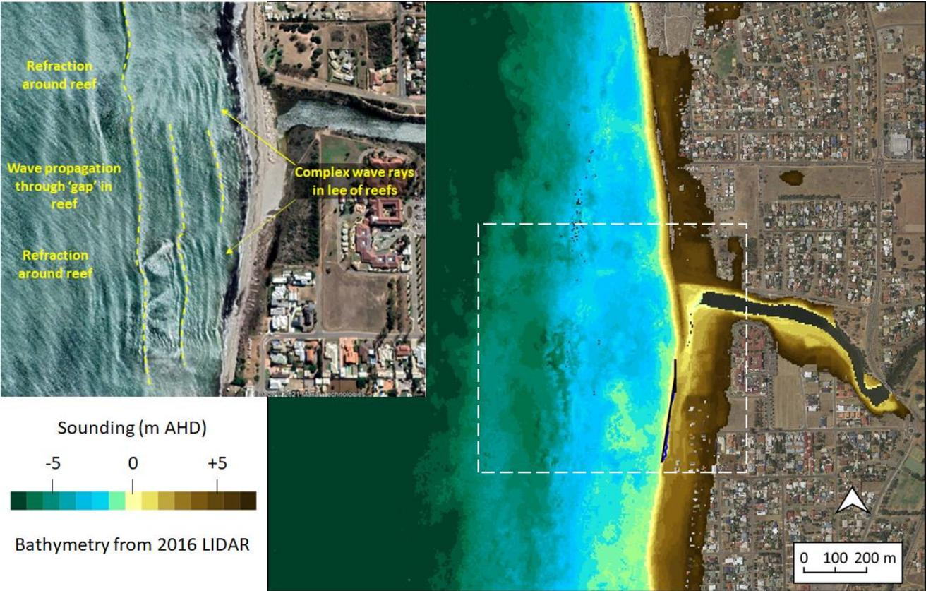
Figure 2-3: Local Bathymetry and Influence of Reefs on Inshore Waves
