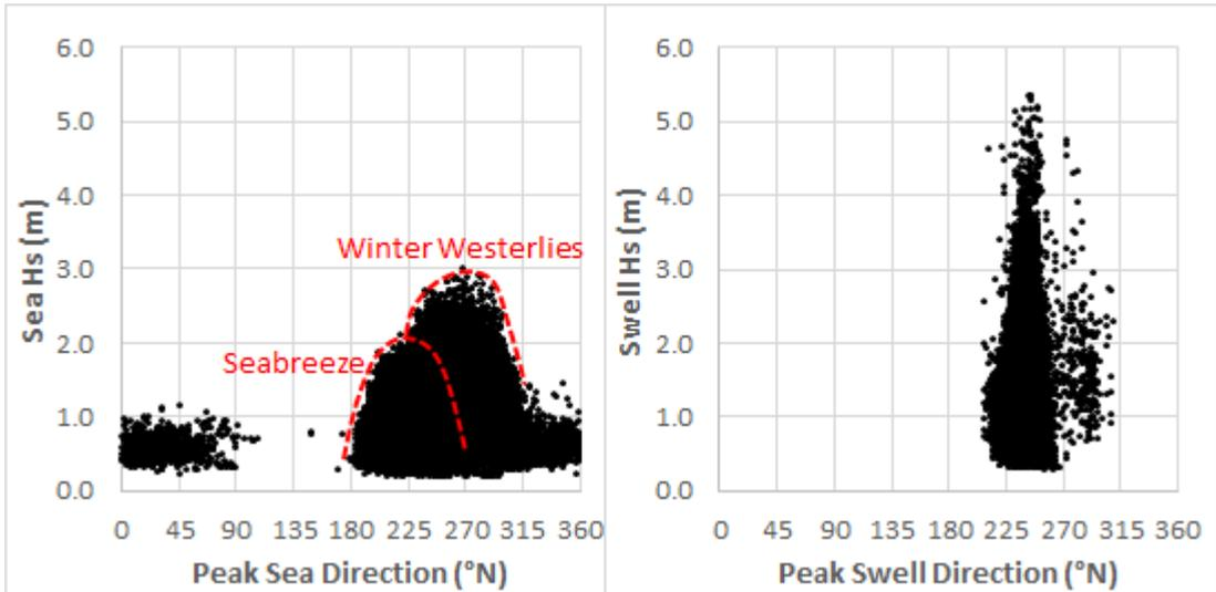
Figure A-8: Sea and Swell Wave Height Versus Direction
