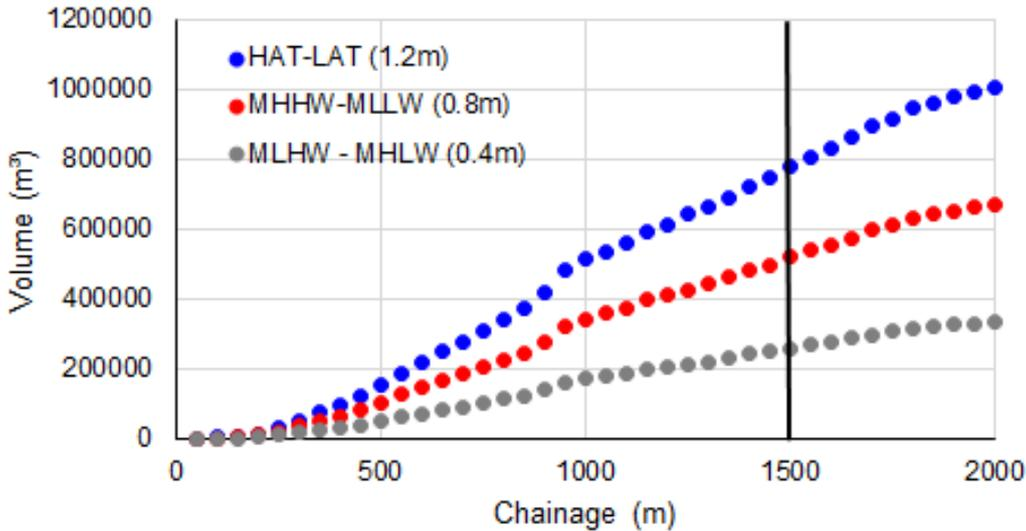
**Figure B-23: Basis for Tidal Exchange (Efficiency  $C_T = 1.0$ )**
