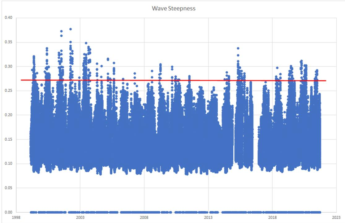
Figure B-21: Wave Steepness Derived from Offshore Wave Time Series
