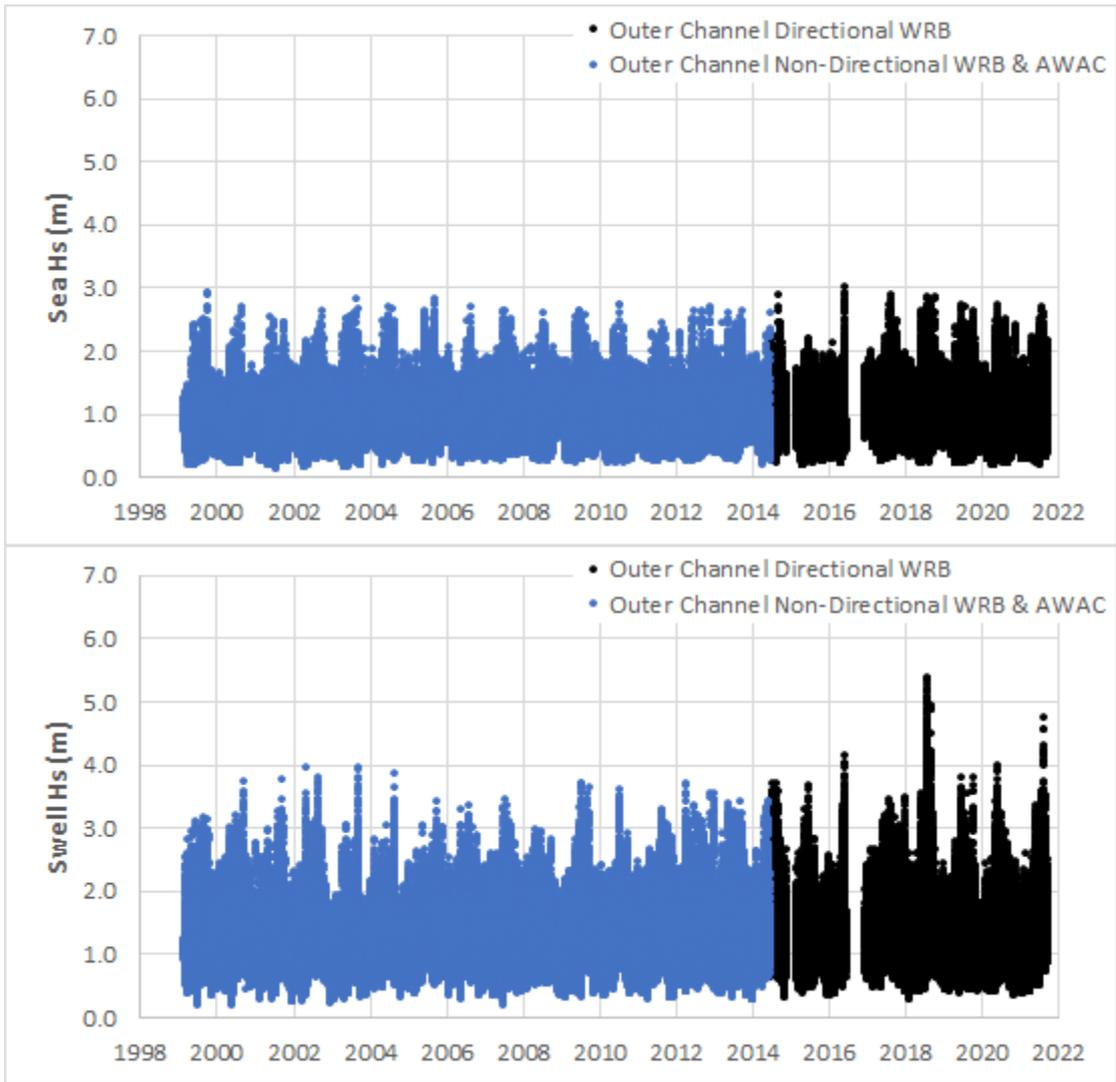
Figure A-7: Timeseries Showing Sea and Swell Wave Heights at Geraldton (Offshore)
