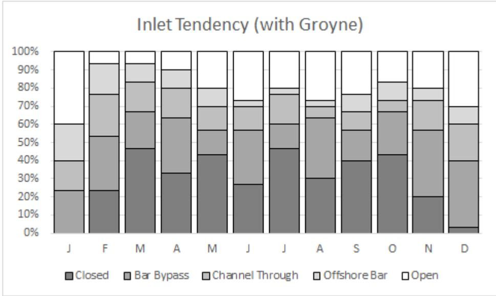
**Figure 3-3: Inlet Tendency Due to Tide and Alongshore Transport with Groyne**
