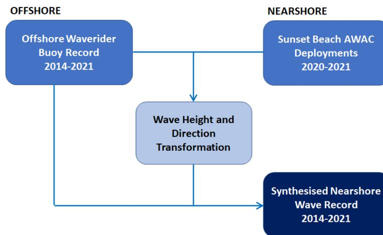
Figure B-6: Schematic for Process of Wave Data Interrogation
