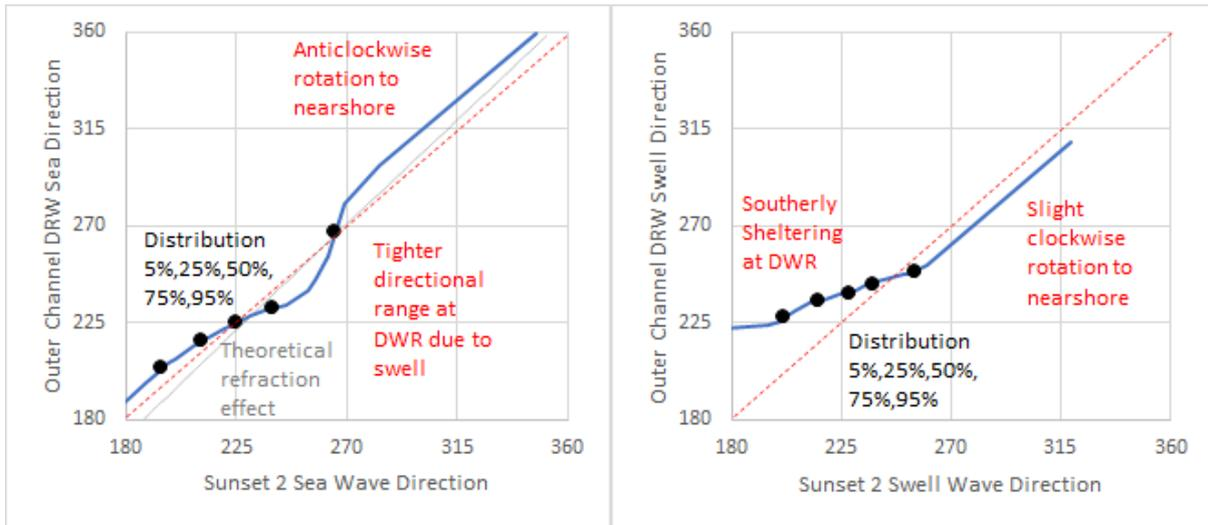
Figure B-8: Comparison of Offshore and Nearshore Wave Direction Distributions
