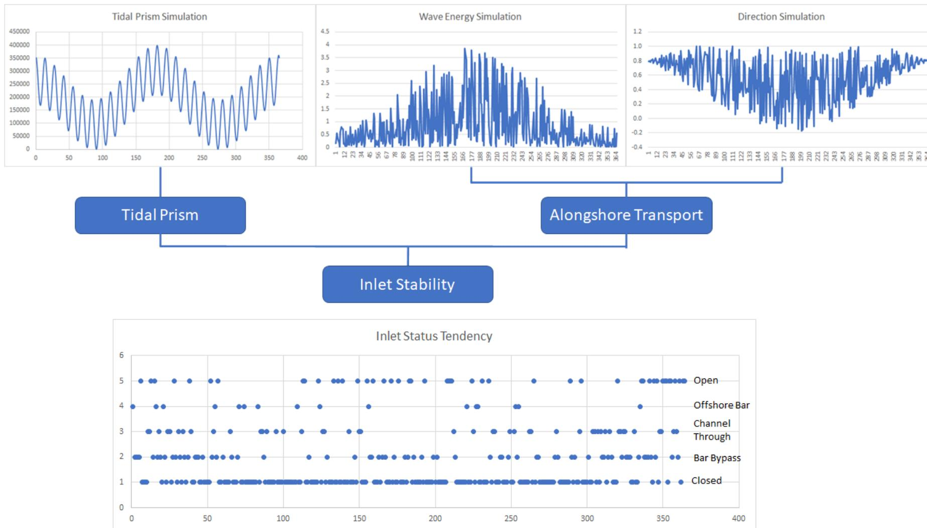
Figure 3-1: Components of Entrance Stability Simulation
