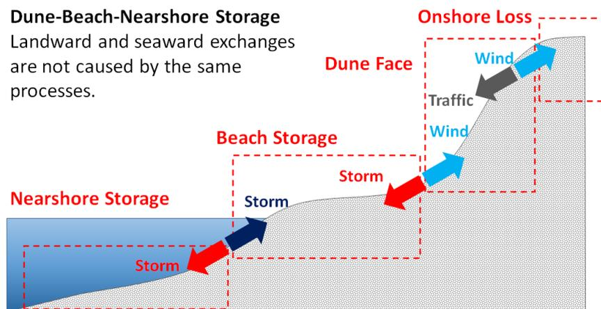
**Figure B-20: Cross-shore Zones and Connections**
