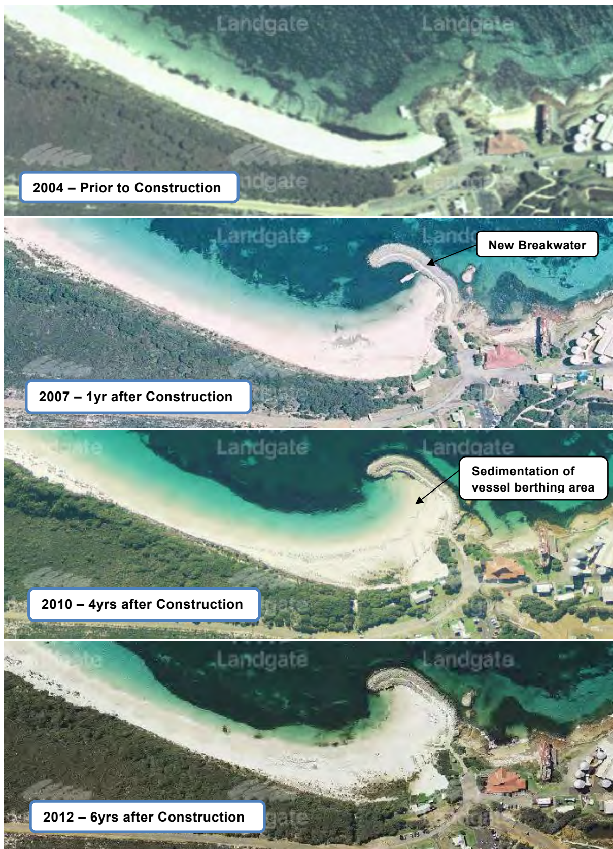
Figure 4.2 Images Showing Change in Beach Alignment behind Whale World Breakwater
