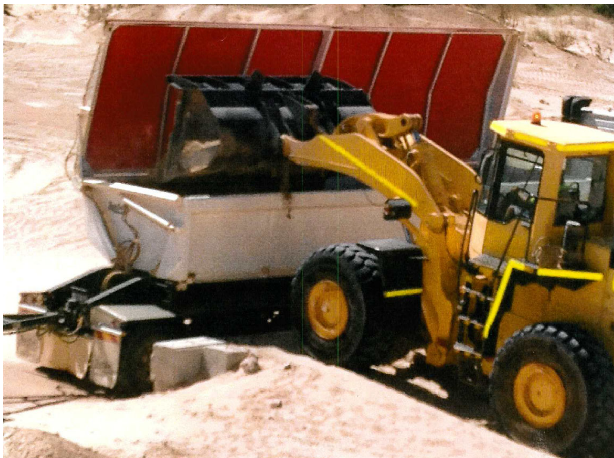
Figure 3.2 Loading Sand Directly into Waiting Road Trains (Mid West Sands)
