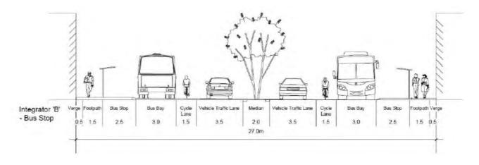
Figure 11a.1 Conceptual Road Cross Sections – Integrator 'A' & Integrator 'B'
