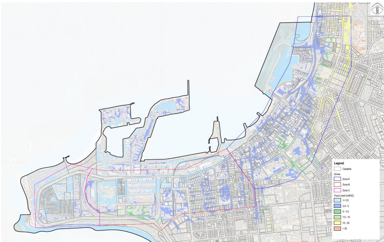
Figure 8-1 Peak rainfall extent 100year ARI (2070) event. High resolution maps provided in Appendix B.
