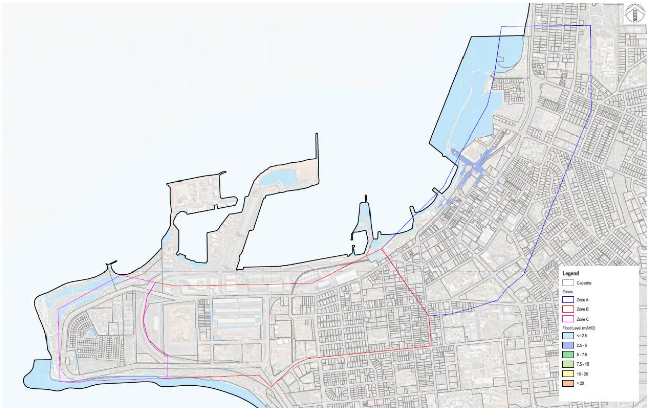
Figure 8-5 Peak Tsunami Extent 500year ARI (2110) event. High resolution maps provided in Appendix B.
