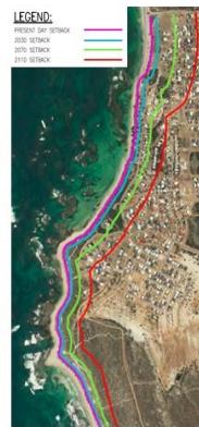
Drummond Cove: Coastal Erosion Setback Lines
