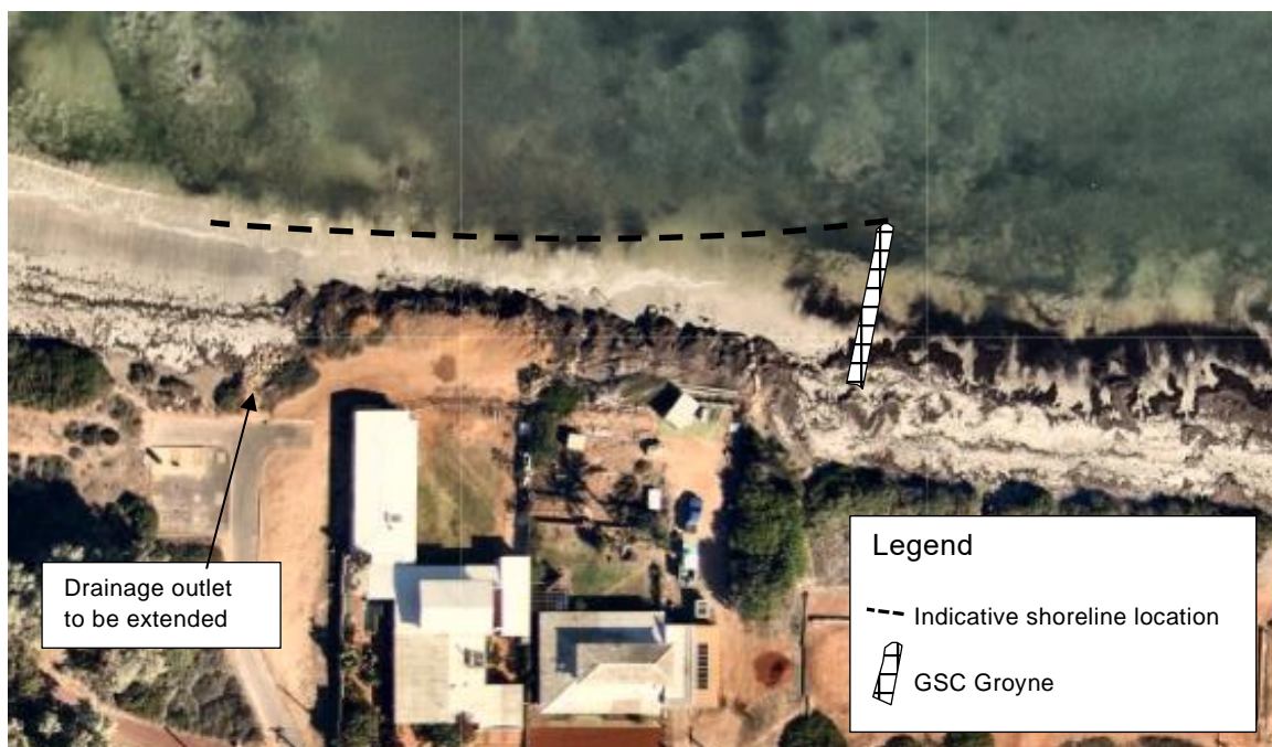
Figure 5.3 Bluff Point North Interim Adaptation – GSC Groyne Option 1
