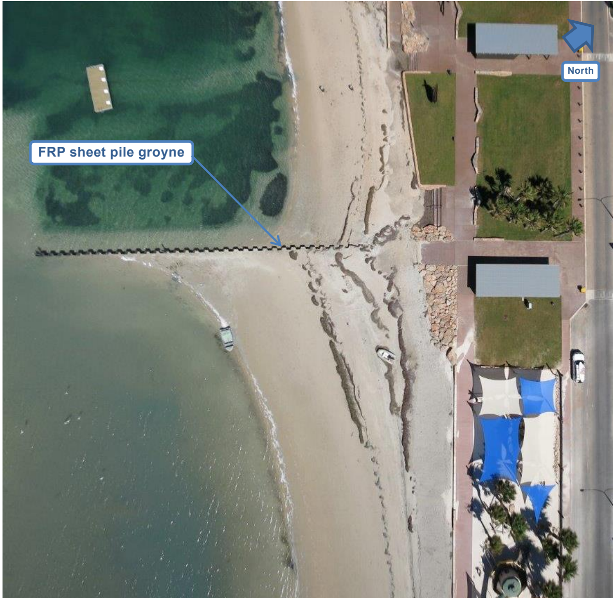
Figure 3.7 Denham Foreshore Composite Sheet Pile Groyne Aerial Photograph (Supplied by Department of Transport, 2016)
