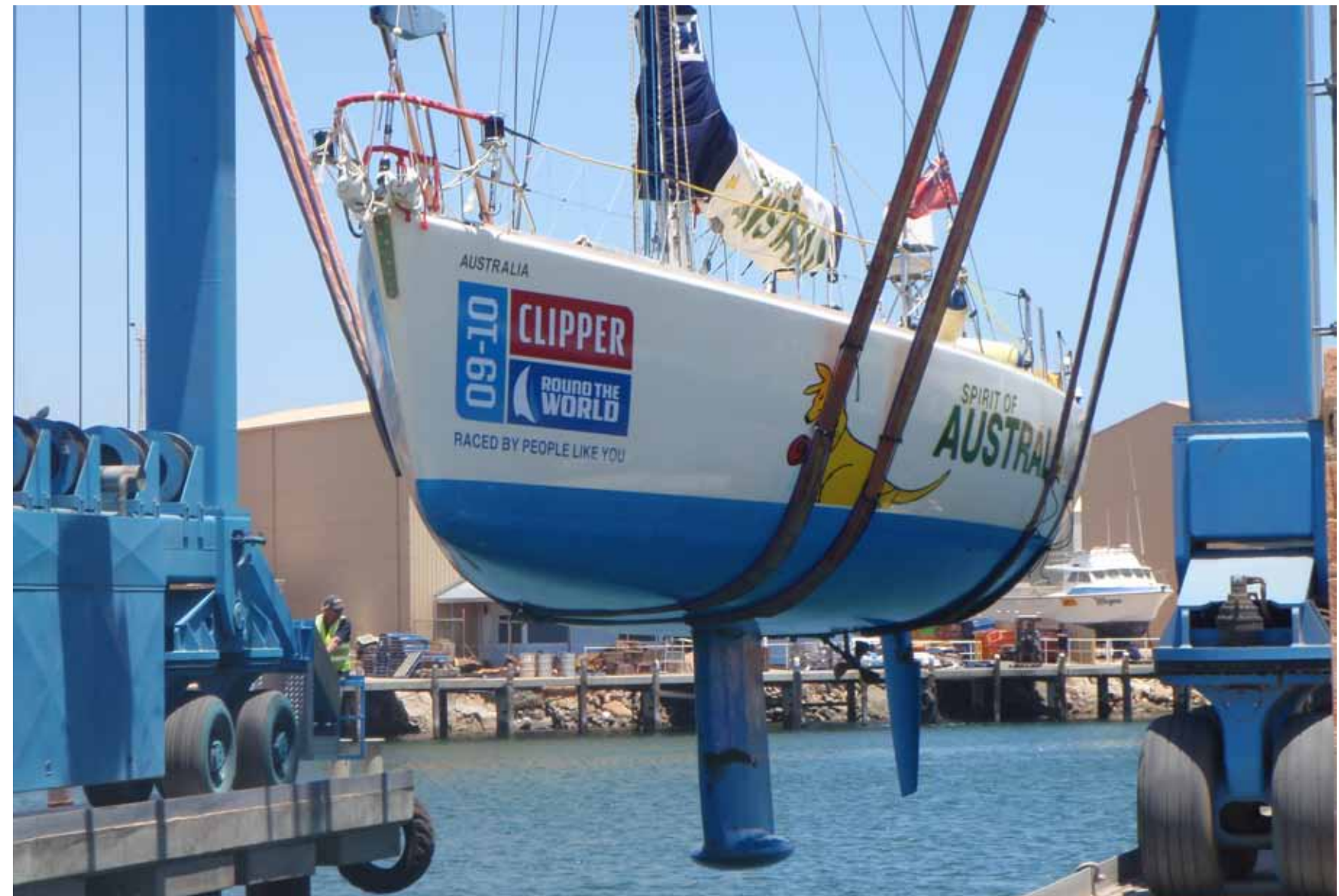
Geraldton Heavy Boat Lifter, taking Spirit of Australia out of the water for service
