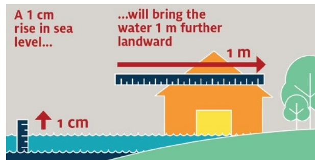
FIGURE 5. SCHEMATIC REPRESENTING THE HORIZONTAL EROSION ALLOWANCE FROM PROJECTED VERTICAL SEA LEVEL RISE - A FACTOR OF 100 (COASTADAPT, 2017)
